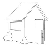
The water heater is to be installed at ground or floor level on a stable fireproof base as acceptable to local authorities. The water heater must also stand vertically upright with the back of the water heater **against or within 25 mm of an external wall** or alternatively against a fireproof screen extending at least 500 mm above, below and either side the flue terminal. Failure to observe this precaution can cause problems in high wind areas.
